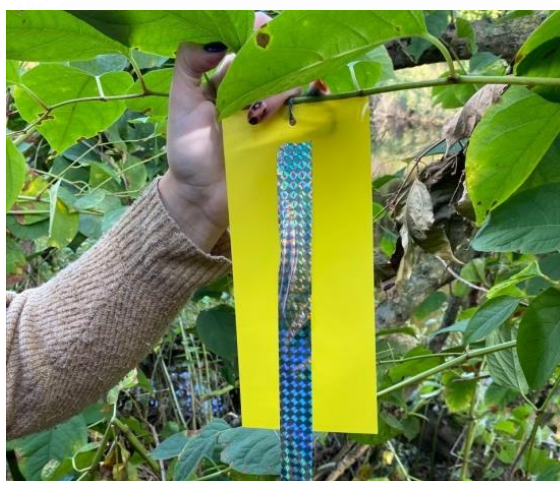
Figure 11. Silver tape attached to centre of sticky trap to deter birds from approaching sticky traps with the aim to reduce the risk of bird mortality from birds getting stuck on the trap
